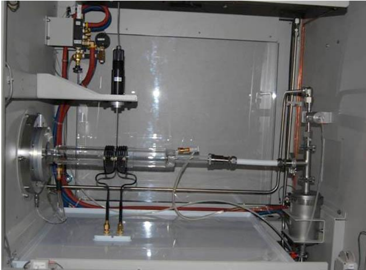
Water cooled, Quartz Process Tube & Optical Pyrometer
